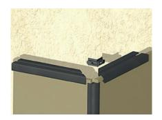
In the same case as step 7, in which the facade does not extend from wall to wall but forms an angle on one side, the two chamfered profiles No 935 of the upper beam are connected between them with the special angle, and the additional transverse leg profile No 935 is screwed onto the HPL sheet, according to the procedure of step 6.
